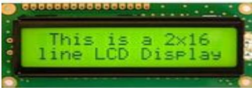
Fig.2. LCD Display
