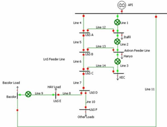
Fig.3. Single Line Diagram of Proposed Reconfiguration
