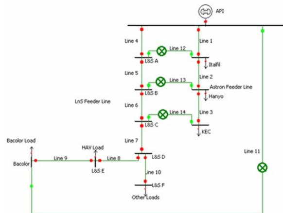
Fig.2. Single Line Diagram of Existing Configuration
