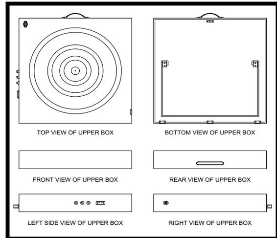
Fig.1. 2D Orthographic View of the Automated IPAD's Top Box
