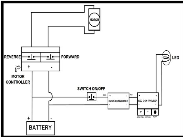
Fig.3. Electrical Circuit Diagram of the Automated Improved (IPAD)
