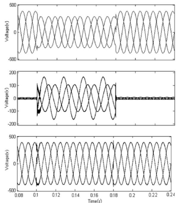
Fig.2. Three-phase voltages sag: (a)-Source voltage, (b)-Injected voltage, (c)-Load voltage
