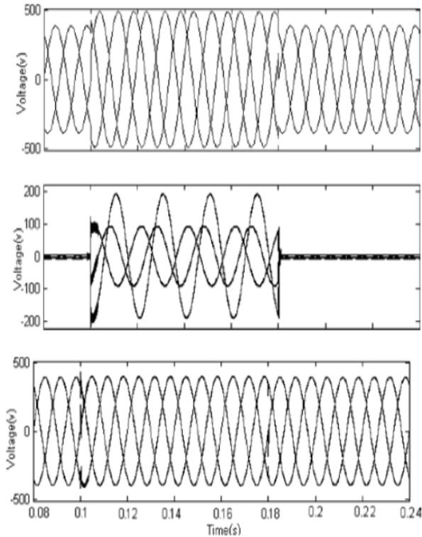
Fig.3. Three-phase voltages swell: (a)-Source voltage, (b)-Injected voltage, (c)-Load voltage
