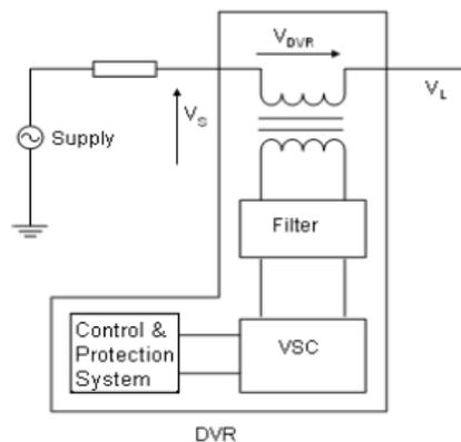
Fig.1. DVR Series Connected Topology
