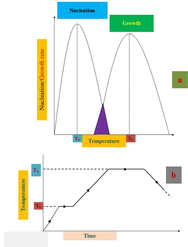
Fig.2. To make a glass-ceramic, glass crystallization used. (a) Temperature affects nucleation and growth rates, with minimal overlap. (b) a two-stage heat treatment
