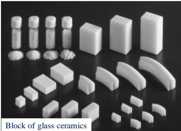
Fig.8. Block glass ceramics for medical applications, as produced in the laboratory
