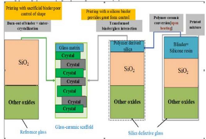
Fig.4. Glass-ceramic processing schemes: traditional devitrification (left) vs heat treatment of silicone/silica-defective glass mixes (right) [48]
